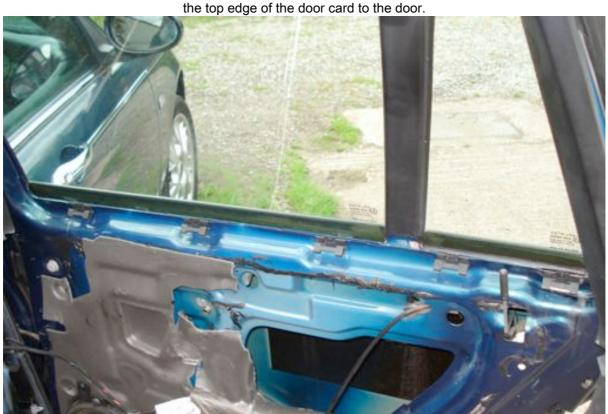
With the clips in place the waist seal is then secured into the clips
