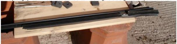
I used a mitre block to cut the leading edge of the seal to the same length of the original
