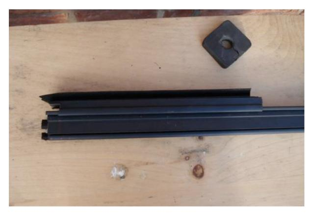
I used the set square to mark the trim lines and then again used the mitre block to acquire a true cutting angle. This resulted in this:
