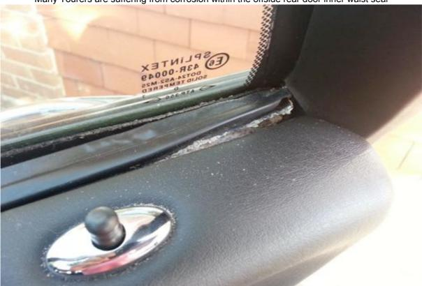
The inner waist seal part number ELT100260 is no longer available. However the inner waist seal for the LWB Limousine is available, part number ELT000060, and can be trimmed to fit the Tourer. Tools required: hacksaw, tee-square, black sealant, rust treatment/inhibitor and mitre box. To start you will need to remove the door card and ease the lower parts of the inner plastic door trim away from the window frame:
