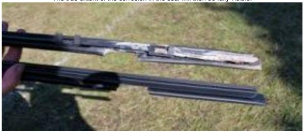
The corrosion extends to the grove cut into the seal for the rear quarter light,
