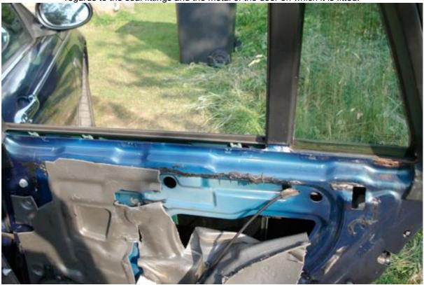
Corrosion has affected the metal of the door where the rear most fixing clip was seated; this was removed and treated with a rust inhibitor. Although the door cards are non-metallic some rust had become encrusted where it met the corroded door metal and clip.
