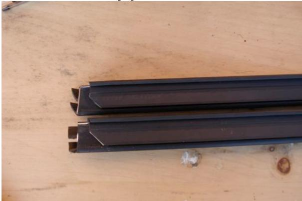
The rubber trim was then cut to match the profile of the original seal as shown below
