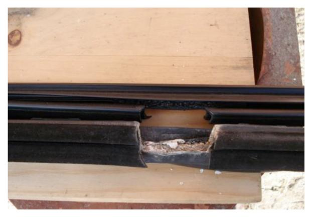
This corrosion is not usually visible when the seal is in place.
