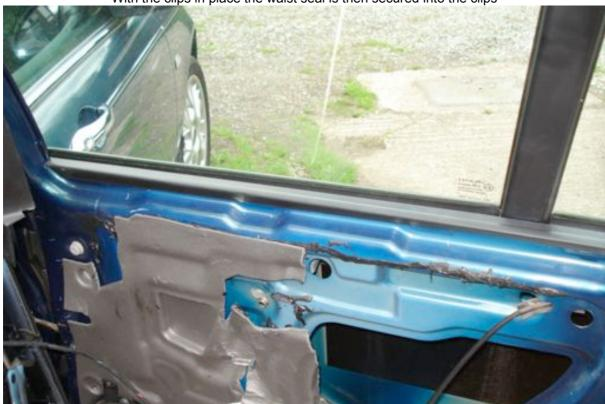
The rear of the seal is a little too short so you will need to cut a piece from the original seal to make up the difference. To prevent rattles I cut a section that could be made secure by applying a bead of black silicone. However I am also using this to monitor what was the most heavily corroded area.
