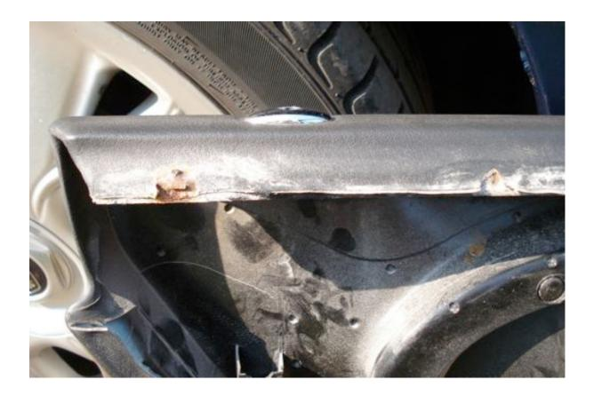
This was removed and a rust inhibitor was brushed onto the affected area. Some of the original clips were reused however one had been completely corroded and another showed slight signs of corrosion so these were replaced with new clips. These clips fix the seal to the door and also secure
