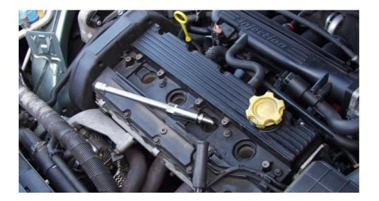
Once you have replaced all the plugs its time to replace all the coil packs and leads, simply move them all back into position as before and place the bolts in the bolt holes on the coil packs
