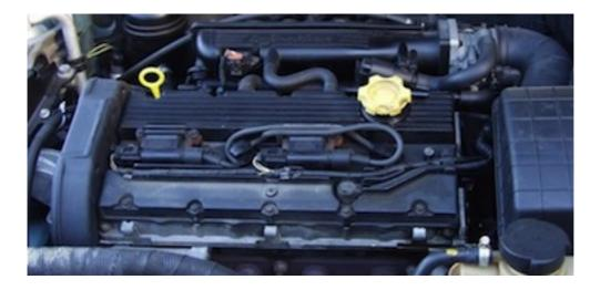
Don't put the spark plug cover on just yet, Start the car up and stand back and admire your work if every thing is ok, then replace the cover, please remember your cover is made of PLASTIC, if you tighten it up too much it will crack, steady as she goes captain.
