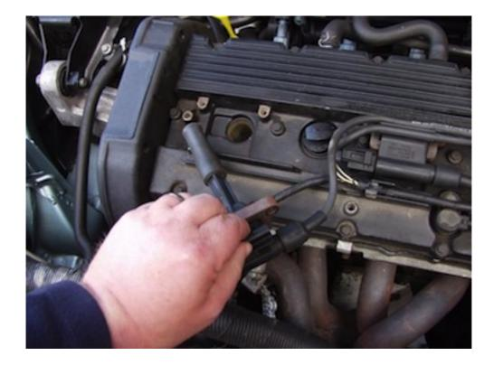
Then place the spark plug socket in the hole and push onto the spark plug, turn the wrench anti clockwise, when it loose you can remove the wrench and simply unscrew by hand using the socket and extension bar, I find this method fasterthe plugs that came out were ok and in good condition.
