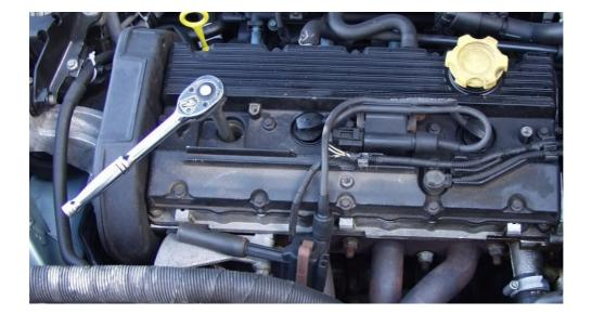
So now you have replace the first one, are you ready to tackle the others, they are just as easy (unless you gave up earlier) You already have one coil pack out, the next lead simply pull out, at this point be careful not top disturb the lead that's are in the guide rails on top of the 2nd coil pack, this is to keep reinstallation easier.
