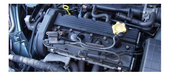
Place the whole set of leads carefully out of the way, be careful not to disturb the order of the leads.
