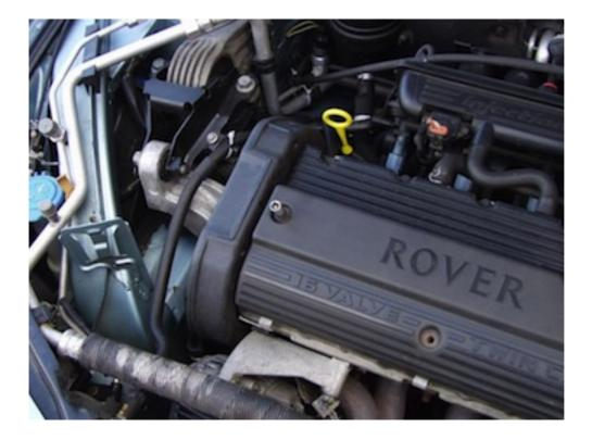
When each bolt is loose pull them out and lift the spark plug cover away. Place the cover upside down and place on a cloth so not to damage it and us this to keep any bolts secure.
