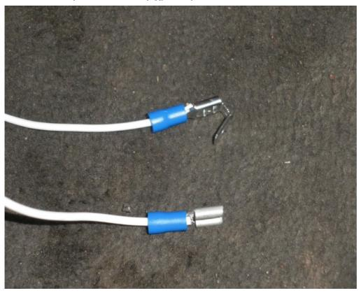
Push the fuse you removed earlier into the female and piggy back connector, thus jointing the wires
