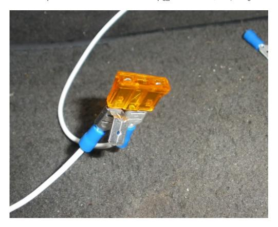
push the male ends into the space in the fuse box where the fuse was removed from
