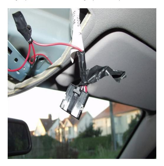
You can place one wire in the connector block and then connect the two live wires from the footwell lights the one wire.
