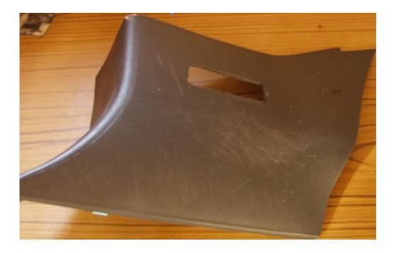
when your light sits in snugly, sand all the plastic bares away and if you are happy with the position of the light, if you notice, on the light there is a clip on one end and guides on the other, the end with the guides needs to be thinner so they slide in place, the clip on the other then can be bulled over the back of the fascia plate, then when it in place, use the hot glue gun to secure it.
