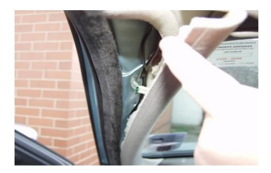
Thread the live wire down the gap at the base of the A pillar, generally the wire will appear at the bottom in the foot well, but some times loses its way, so try again, a little patients is needed here.
