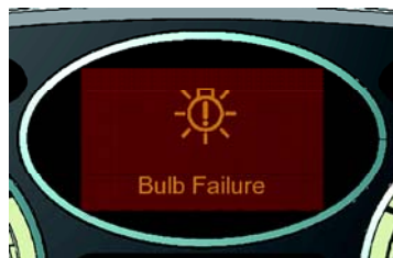
Figure 45: Bulb failure warning lamp
