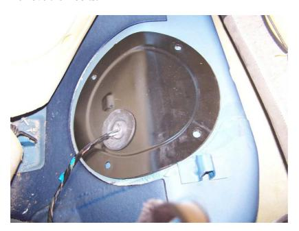
Pop out the large grommet from the cover plate so you can move it out of the way without disturbing any cables.
