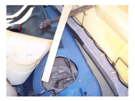
Now you can lift out the pump, it's a bit fiddly and the long wire and float for the fuel level mechanism needs to be wiggled about to come out.
