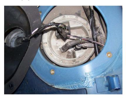
Do retest to make sure the car starts and runs Bolt back the cover plate and reseal the large grommet. Put back sound proofing, carpets, and the seat base. Those rear wires will be little monkeys;-)
