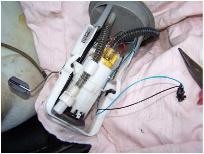
You now have to separate the pump section from the main section. Does this by pulling out the 3 black rubber pieces with a pair of pliers.
