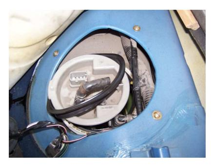
Refit the threaded ring, don't force it, it will fit easily a screw on finger tight. Then tap tighten with the wood and hammer/mallet.
