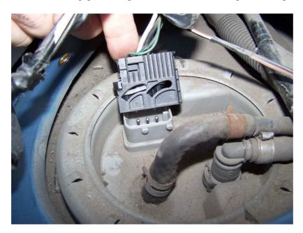
You will see the access cover to the tank held on by a large threaded ring. Using a piece of wood and the hammer/mallet on the many raised lugs, Tap the ring anticlockwise and unscrew. It Move the ring out of the way,
