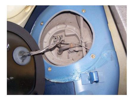
On the top are the electrical connector, and 2 pipes. (Feed and return, I think!) The connector is removed by pulling the outside one way; it should automatically jack the plug off. You can see from the photo the jacking slots and lugs .Remove the 2 pipes & clips. The lower one has a push in clip fitting .
