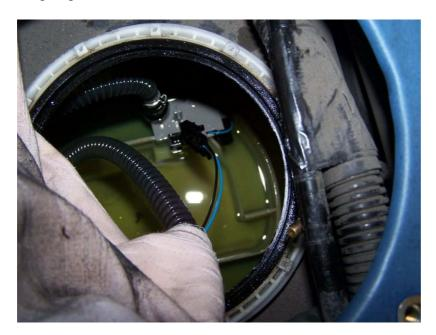
There is also a large rubber seal in the tank opening, try not to lose it down in the tank.
