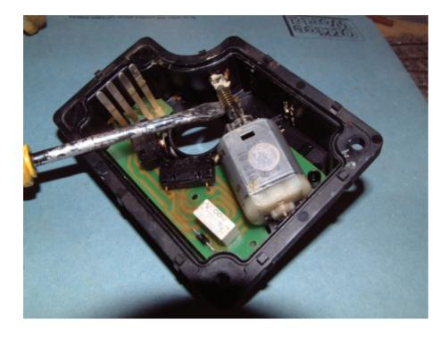
At this stage the switch terminals can just be re soldered and the actuator put back together, only to fail again. You can improve matters by screwing the switches down. You will need a 1,8mm drill, 8BA tap and 8BA by 1/4 inch screws. Or use 2mm if you prefer metric! These can all be obtained from
