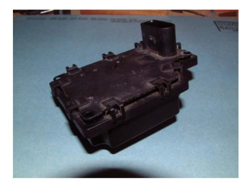
Cut a suitable piece of wood or metal to fit right inside the electrical connector
