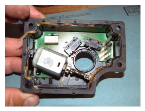
One or both of the two black limit switches is likely to be loose. This is due to poor location resulting in broken soldered joints. The next stage is to remove the circuit board. First, prise out the worm. Take care not to loose the washer off the end of the worm shaft. Use a wide flat blade to spread the load and unclip the worm, bringing the motor and PCB with it.
