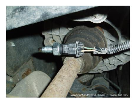
At this point, I looped the plug to check that the lights worked and the switch was faulty. Don't forget to turn the ignition on to check.
