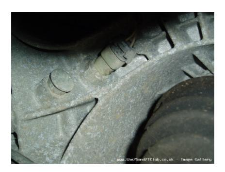
19mm deep socket and the old switch is removed.
