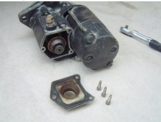
The solenoid can be drawn out of its housing taking care not to lose the spring
