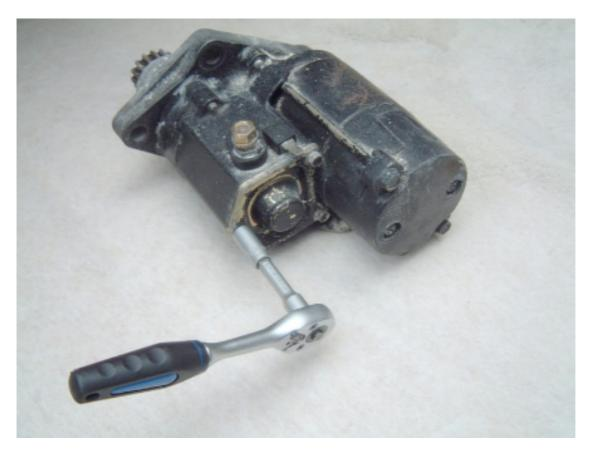
These bolts secure the cover plate that houses the solenoid. There is minimum pressure applied to this plate by the solenoid so although care should be taken, things are not going to fly all over when you remove it.
