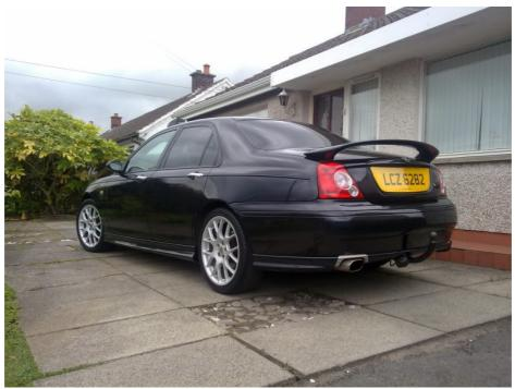
The single bodykit options for the cars where a set of side skirts/sill covers and rear "spats" which wraped around the rear bumper, you can clearly see them along the bottom areas of the car.
