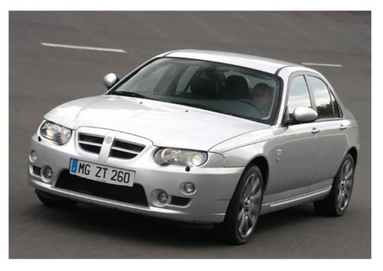
The body shell and chassis of the car was almost identical to the Rover 75, but with more aggressive grille, sportier styling, stiffer suspension and re-tuned engines, along with a more interesting advertising scheme.
