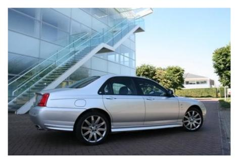
Also on this silver car is the smaller spoiler fitted to the mk2 ZT's as standard. Some late mk1's also had this fitted.
