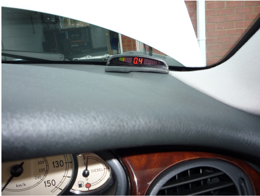
Reversing Sensor Display, indicating an obstacle 0.4 of metre to the nearside rear.
