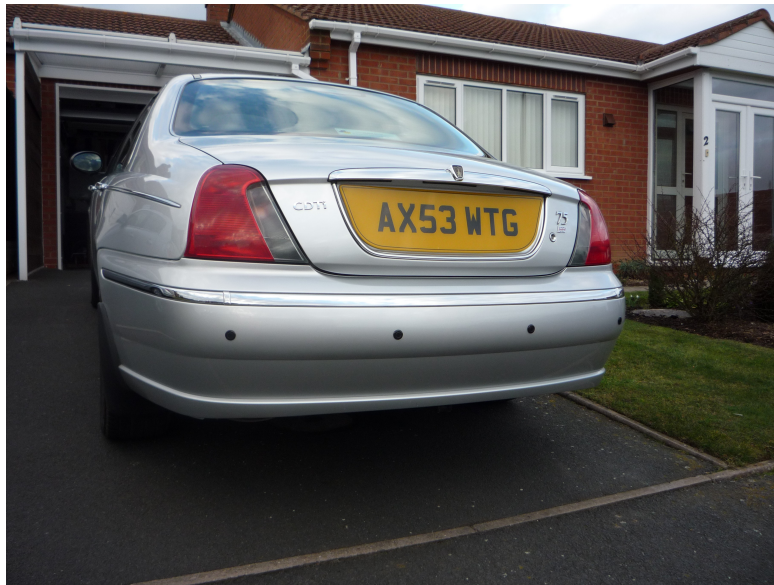
'Maplin' Reversing Sensors fitted to rear bumper.
