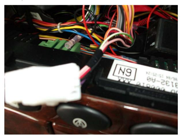
Identify the Light green / White and White / Orange wires at the back of the connector.
