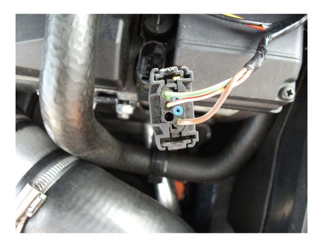
Next, you need to terminate the FBH end of the wire you fed through with an appropriate contact. The genuine Rover contacts are difficult to find but Radiospares do a perfectly acceptable alternative under the part number:- 495-9653 (pack of 100).
