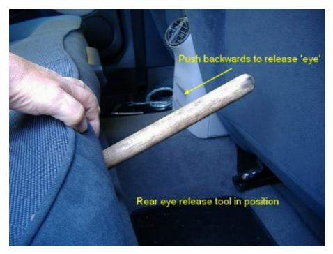
A simple rearward push on the tool while lifting the end of the cushion releases the fastening. Repeat at other side and the cushion can be lifted off the floor.
