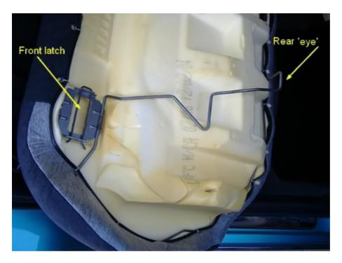
To release the wire 'eye' a long tool of some sort would do a much better job. For my second go, I used a long screwdriver to push the eye backwards off the floor hook. You can lift the cushion just enough to see what you're doing, but it's still frustrating because it slips off the wire. A much better tool is about two feet of old broom handle. I trimmed the end with a hacksaw to give a nicely fitting socket.
