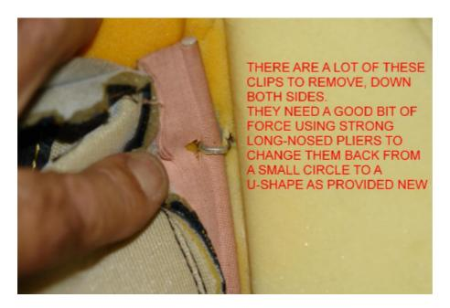
These clips on mine were obviously done using a nice Rover Special Tool. I used two large strong pairs of long-nosed pliers to open them up and remove them. When you have them all out, CAREFULLY remove the cover as before.
