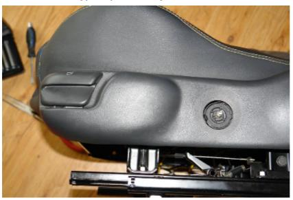
Recline the backrest FULLY and remove the two torx screws shown:
