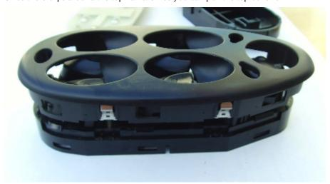
3. Lift the switch unit housing out and put to one side
