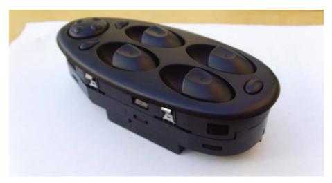
These units can tend to fail with age, normally at the mirror control unit when the 8 - way control button fails to respond and the mirrors don't move.
