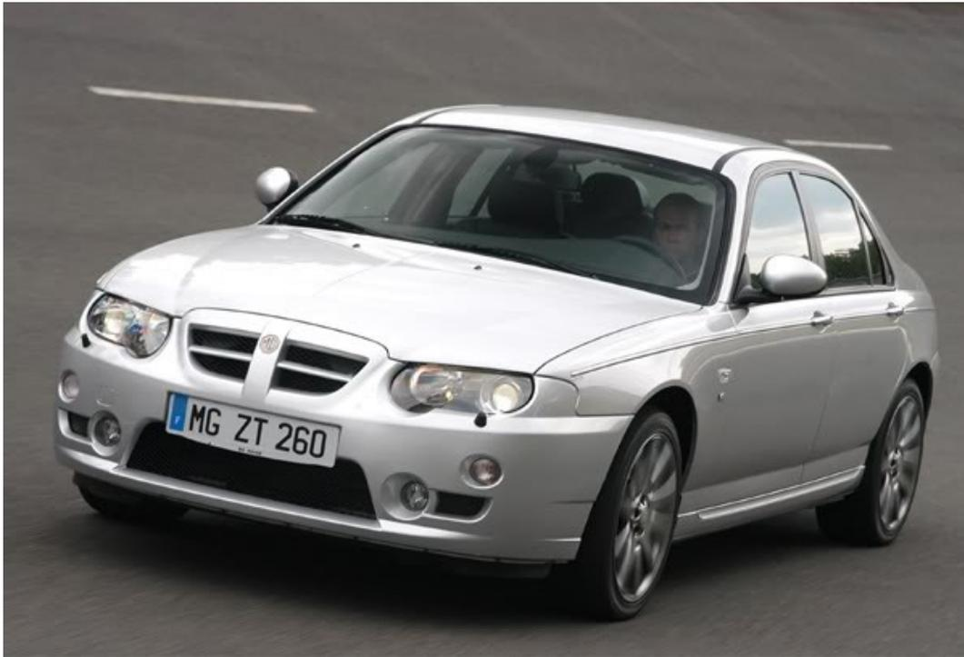
The body shell and chassis of the car was almost identical to the Rover 75, but with more aggressive grille, sportier styling, stiffer suspension and re-tuned engines, along with a more interesting advertising scheme.
