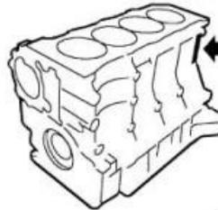
Engine Identification No. location on the K1.8 cylinder block
