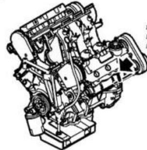
Engine Identification No. location on the KV6 cylinder block
