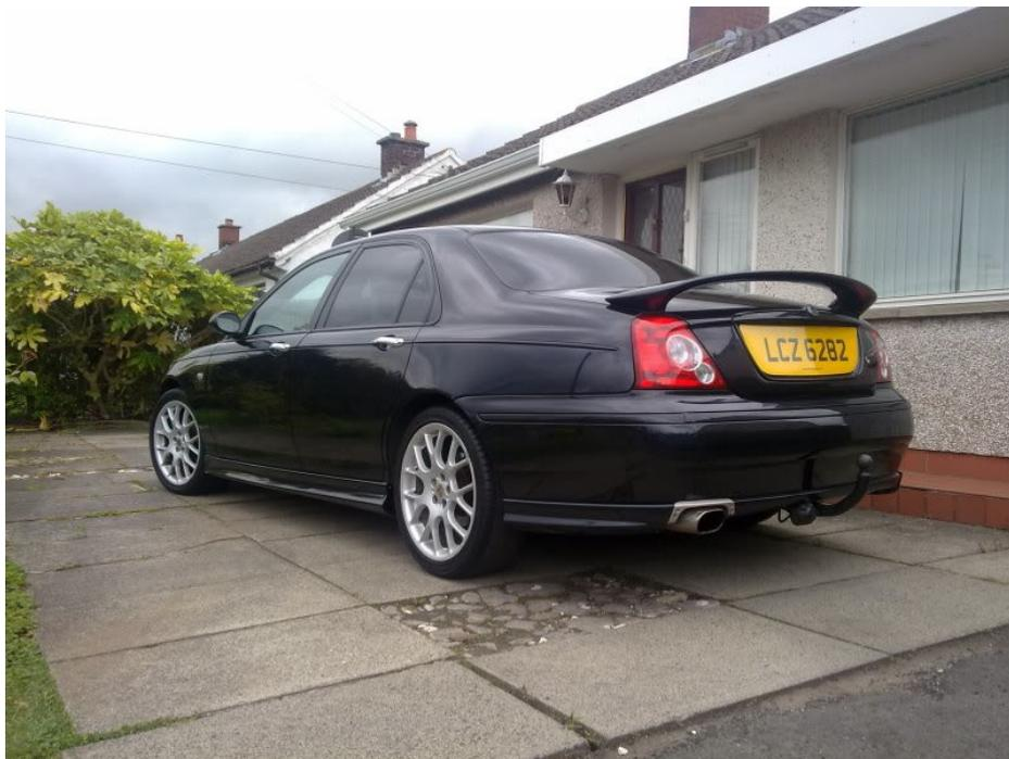
The single bodykit options for the cars were a set of side skirts/sill covers and rear "spats" which wrapped around the rear bumper, you can clearly see them along the bottom areas of the car.
