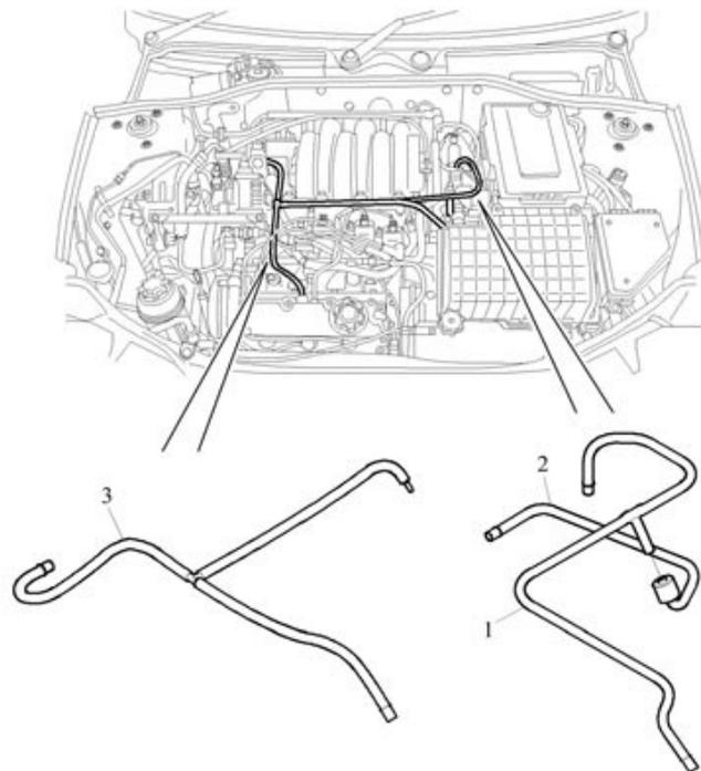
It should be noted that pipe "3" often breaks at the T junction and should be replaced completely, or if your cheap like me, scrape out the inside of the plastic from the three pipes and use a copper T piece from your local B and Q. 22,000 miles later and mine's still fine.
