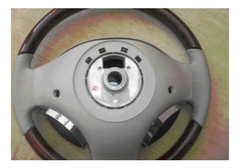
5. Carefully remove the yellow/blue connector from the air bag - this is done by un-clipping the yellow section so it can just pull out. Store the air bag safely facing up.
