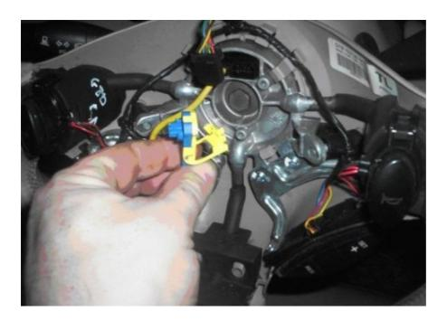
6. Unplug the multi connector from the top of the steering wheel - again this is a clip in connector and comes off easily. This connector carries the connections for the horn and radio controls, as well as cruise if fitted.
